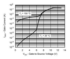
Gate-Current vs. Gate-Source Voltage
