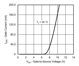
Gate-Current vs. Gate-Source Voltage
