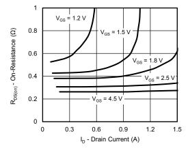
On-Resistance vs. Drain Current and Gate Voltage
