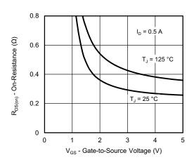
On-Resistance vs. Gate-to-Source Voltage
