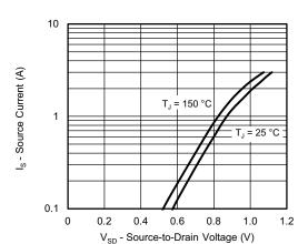
Source-Drain Diode Forward Voltage
