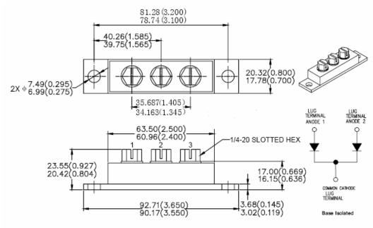
Please Note: Anode 1 = Terminal 1; Anode 2 = Terminal 3; Common Cathode = Terminal 2 Suffix R Denotes for Reversed Polarity.
